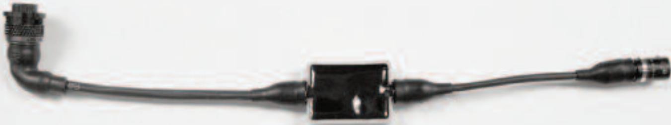
ABOVE MagCanica's signal-conditioning circuit for its new KERS torque sensor system. The unit provides a 0-5 Volt analogue output
